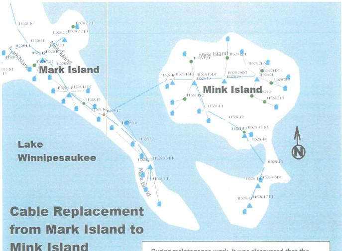
During maintenance work, it was discovered that the neutral wire of the submarine cable feeding from Mark Island to Mink Island was deteriorating and the entire run of cable will need to be replaced.
